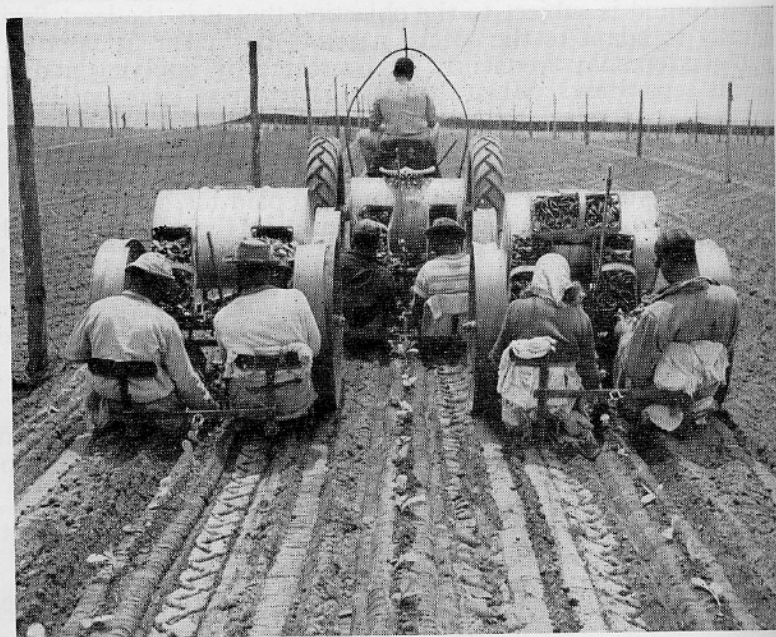
Figure 11. Three-row transplanter at work. (Photograph courtesy of The Shade Tobacco Growers Agricultural Association, Inc.)
