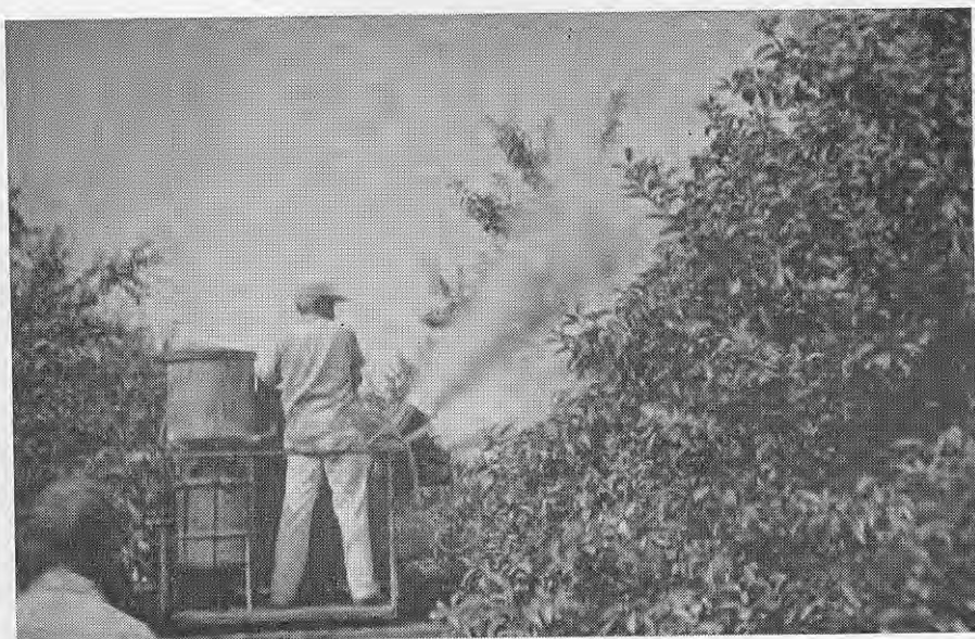
Figure 8. Type of mist blower used in orchard experiments.
