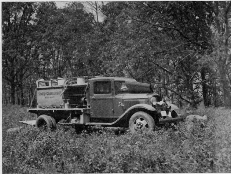
FIGURE 94. This new Fitzhenry-Guptill power sprayer with Ford chassis supplies 1000 lbs. pressure at the engine.
