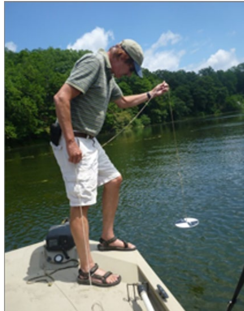
Figure 3. Checking water clarity with Secchi disk.
