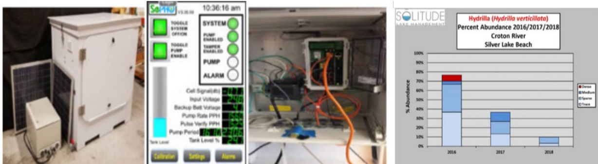
Figure 15. Herbicide injection system successfully used on the Croton River to control hydrilla (photo credit New York Department of Environmental Conservation).
