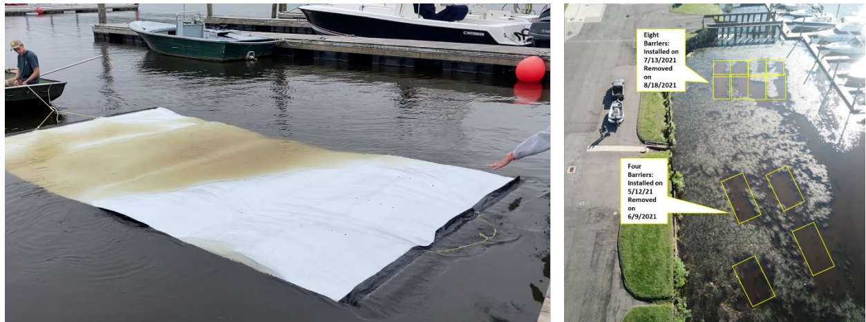
Figure 16. CAES IAPP testing of short-term benthic barriers on the Connecticut River at Portland Boat Works.
