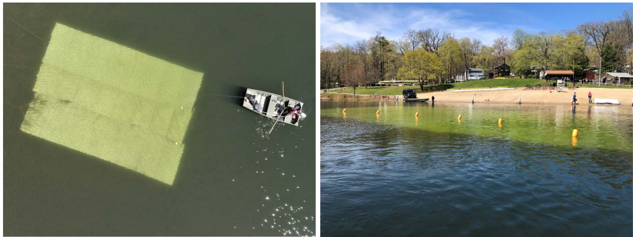
Figure 10. CAES IAPP testing of short-term benthic barriers in Lake Beseck.
