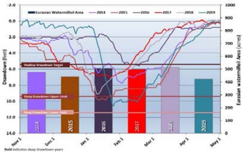
Figure 10. Candlewood Lake’s drawdown depths and duration and Eurasian watermilfoil coverage from 2007 - 2019. Bars with years in bold are deep drawdown years.
