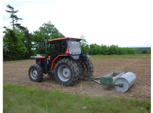
Above: Compacting the soil with a tractor-pulled weighted roller. Photo courtesy of Audrey Maddox.
