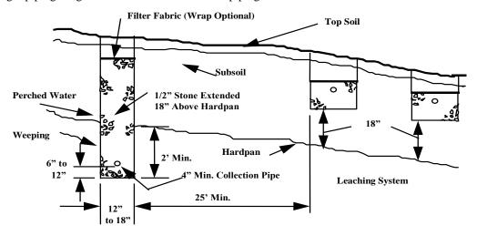
Figure 17 - Typical Curtain Drain Construction
