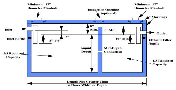
Figure 4 – Typical Septic Tank
