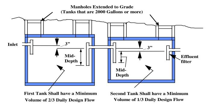
Figure 5 – Septic Tanks in Series
