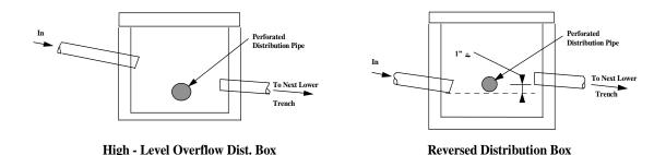
The high-level overflow invert elevation shall be set within the top 3 inches of the upper leaching system row. In order to ensure adequate gas transfer, the use of reversed distribution boxes should be avoided.
