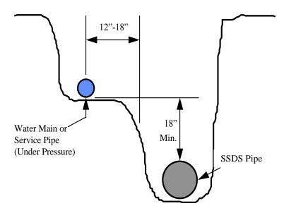
Figure 2 - Pressurized Water Pipe and SSDS Pipe Trenches
