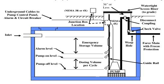
Figure 11 - Pump Chamber
