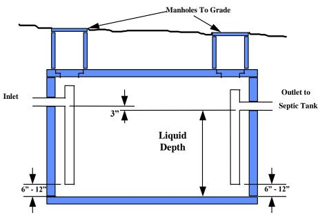
Figure 7 - Grease Interceptor Tank
