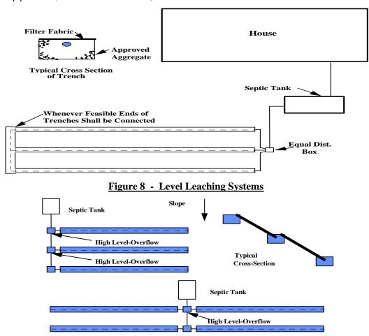
Figure 9 - Serial Distribution Systems
