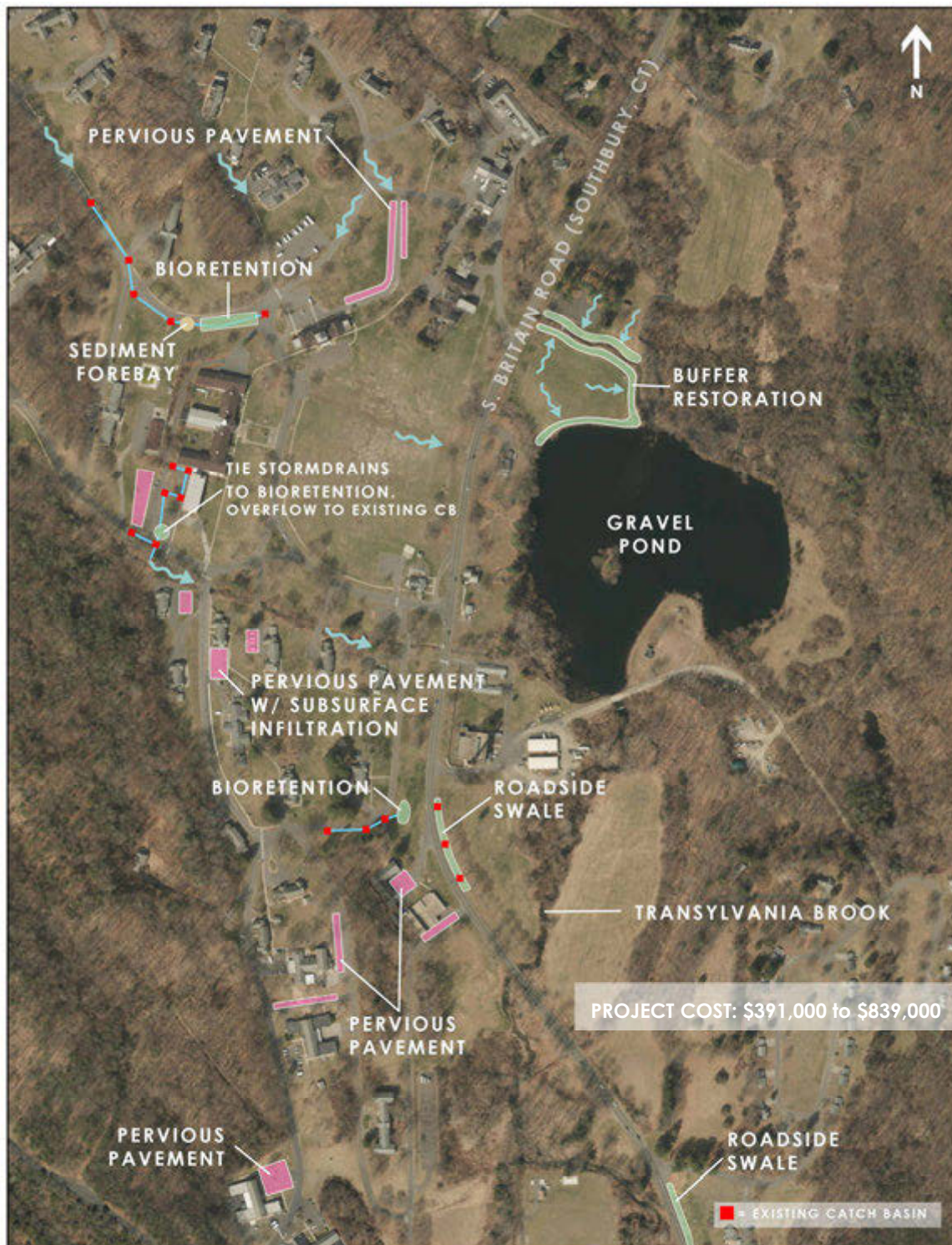
Figure 4-12. BMP Concept: State Facility 2
