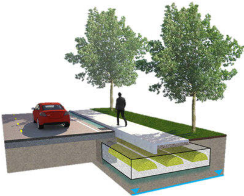
Figure 4-3. Examples of subsurface infiltration systems for parking lots (top) and within the road right-of-way (middle and bottom)
