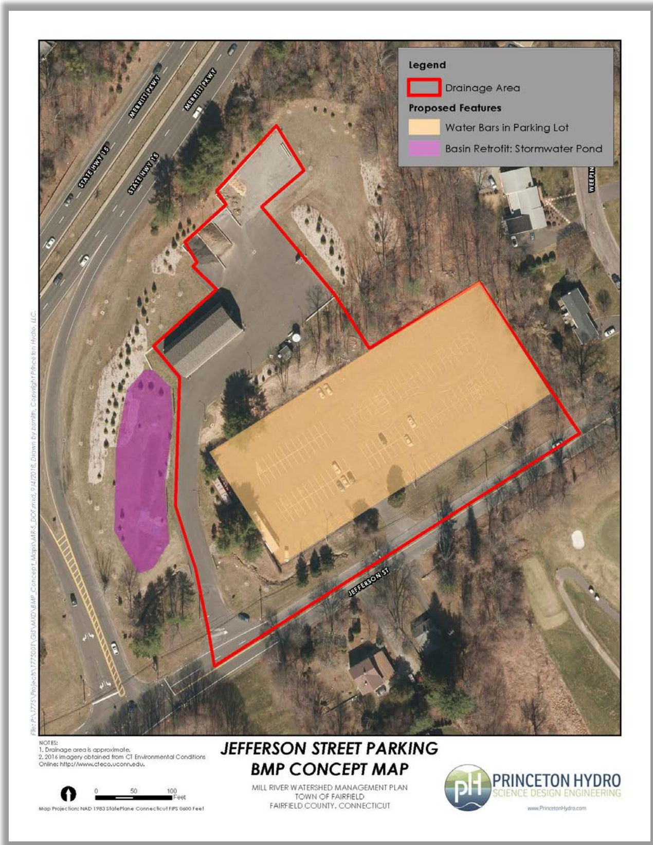
Figure 5.33: Jefferson Street Parking BMPs
