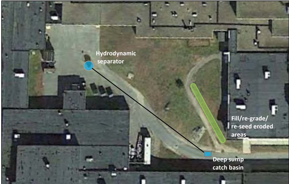
Figure 8-38. Erosion and sediment deposition along a walkway and the edge of the driveway at the Thompson Middle School delivery area (Google Earth imagery dated 10/10/16).
