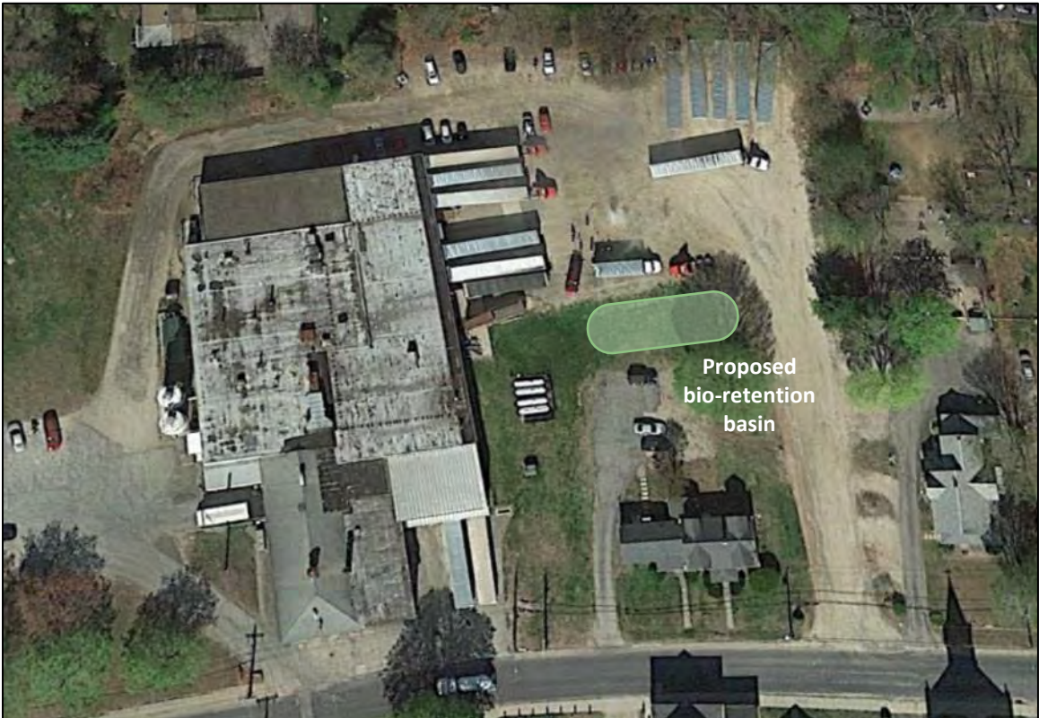
Figure 8-14. Aerial view of the Superior Bakery property on Main Street in North Grosvenordale, CT. Stormwater flow paths can be seen in the dirt parking lot and driveway (Google Earth imagery date 5/6/15).
