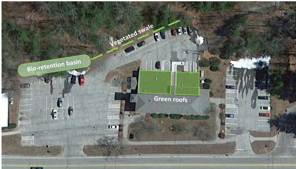
Figure 8-26. Locations of proposed BMPs at the Thompson Town Hall (Google Earth imagery dated 4/7/13).
