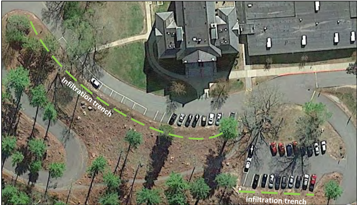
Figure 8-36. Proposed infiltration trenches along parking areas by the Administrative Building (Google Earth imagery dated 5/6/15).
