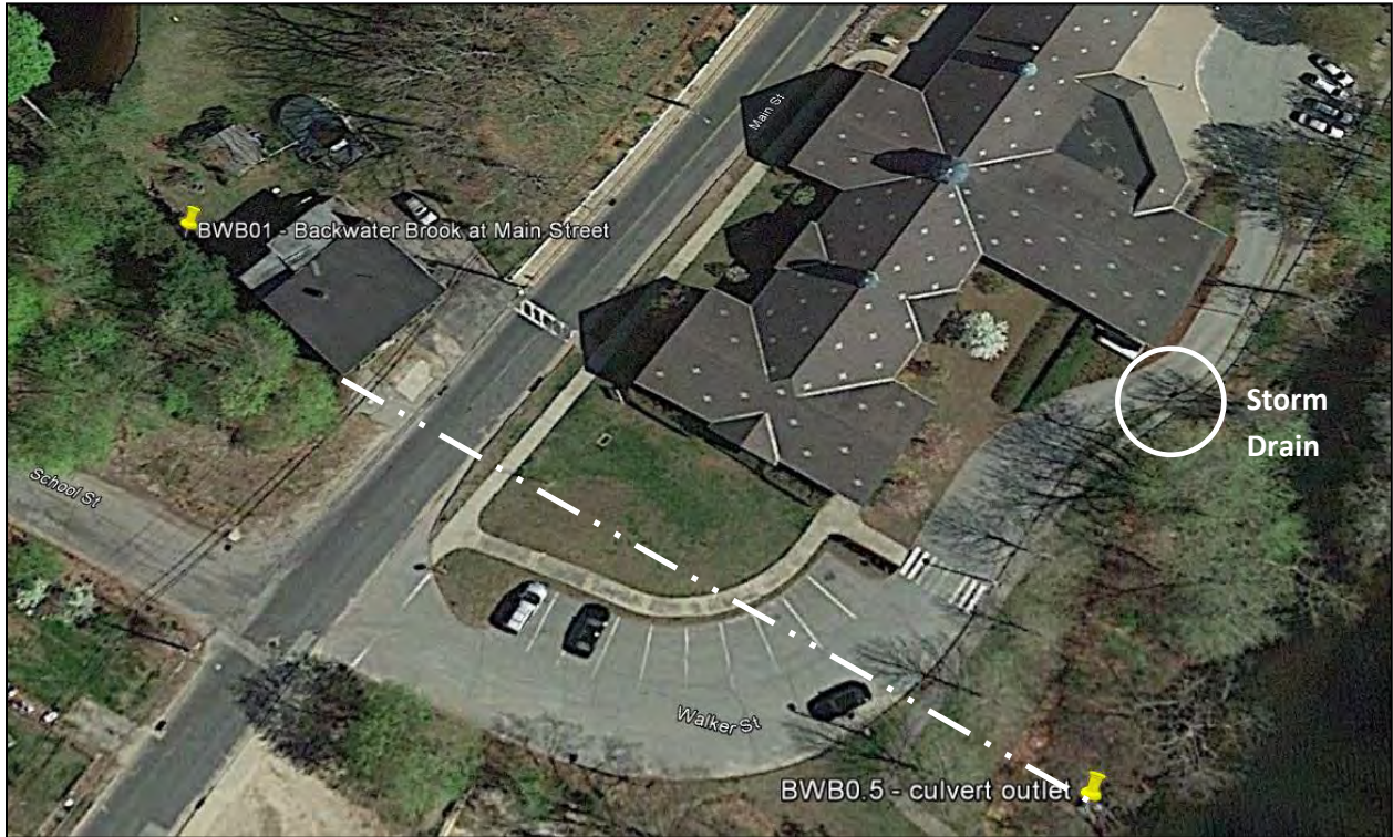
Figure 6. Culverted segment of Backwater Brook (dashed line). Approximately 250 feet of the stream is culverted under Main Street and the Thompson Public Library property.
