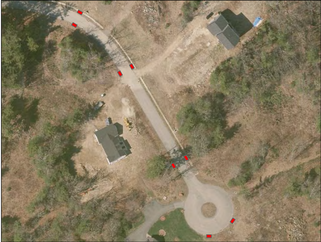
Figure 8-6. The red rectangles depict potential locations of tree filters on Heritage Circle.
