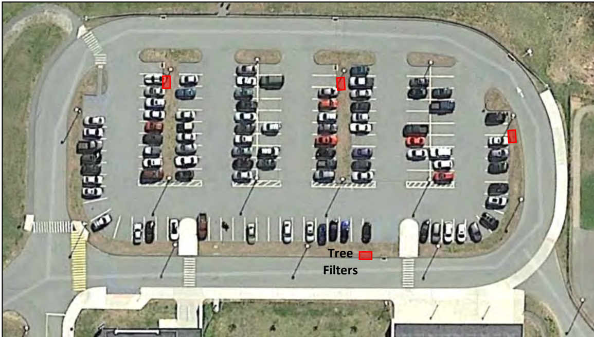
Figure 8-31. Proposed BMPs in the Tourtellotte Memorial High School parking lot (Google Earth imagery dated 5/6/16).
