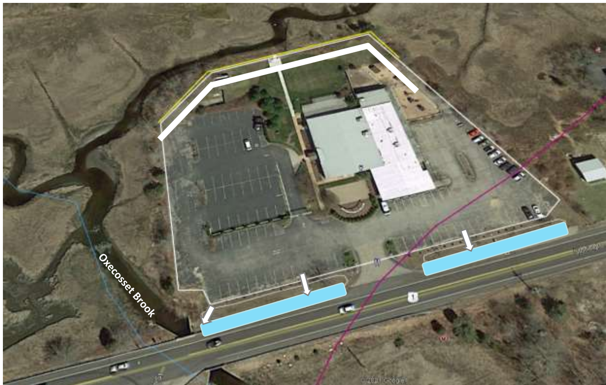
Figure 7-13. The Meadows Event Center in Stonington, CT (Google Earth, imagery date 4/22/2018). The proposed riparian buffer is depicted by the yellow line along the rear of the parcel. The thick white line depicts the proposed permeable reactive barrier. The proposed bio-retention basins are depicted by the blue rectangles. The white arrows depict the locations of asphalt leak-offs from the parking lot. The left-most leak-off presently discharges directly to the brook.
