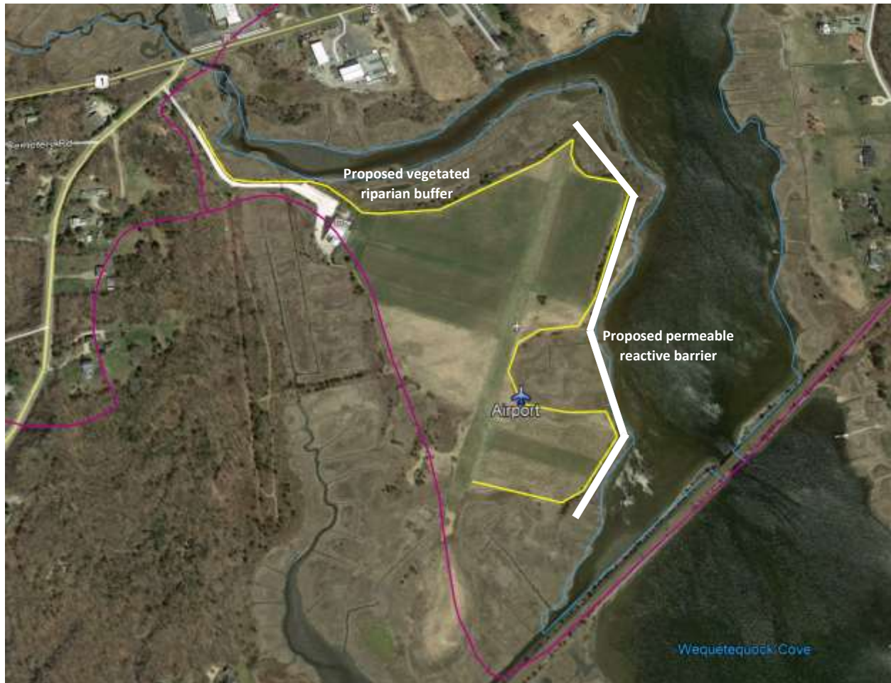
Figure 7-12. Saltwater Farm Vineyard, along the shore of Inner Wequetequock Cove in Stonington, CT (Google Earth, imagery date 4/22/2018). The yellow line represents the proposed riparian buffer restoration area. The thick white line represents the proposed PRB.
