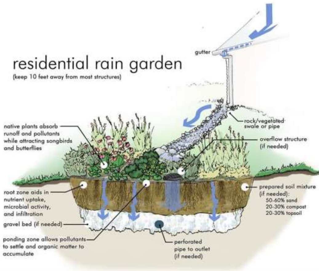
Figure 7-8. Schematic of a residential rain garden catching rain water from a house roof (Image www.500eco.com ).
