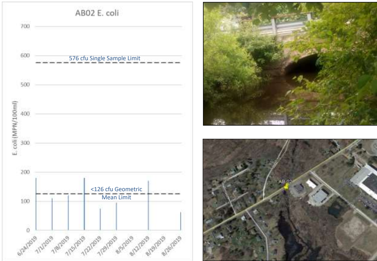
Figure 10. Graph of bacteria sampling results at AB02; upstream view of Anguilla Brook (towards RT 1) at the sampling location; and an aerial image of the sampling site location and vicinity.
