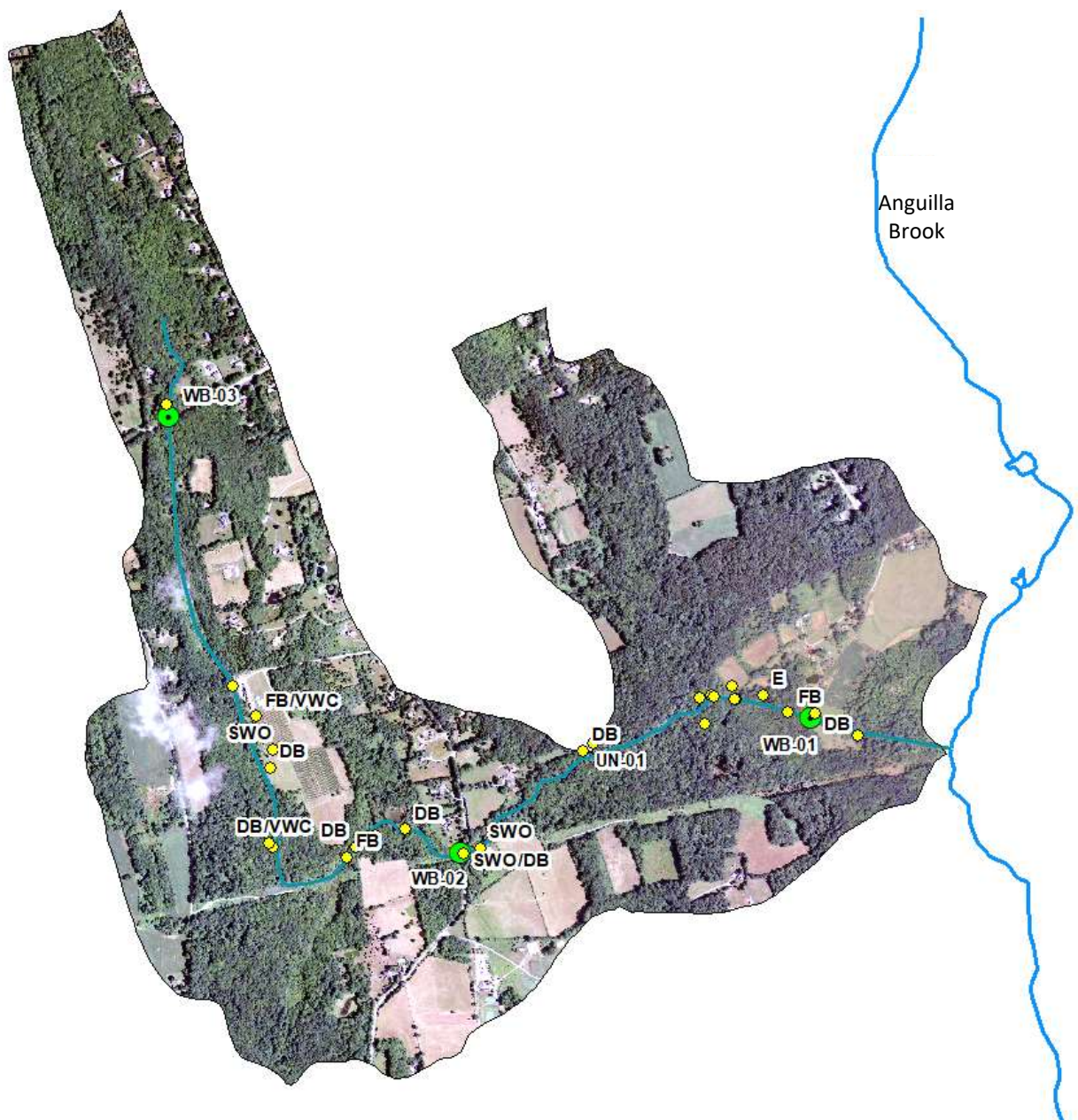
Figure 7. Stream corridor Areas of Concern (yellow markers) identified and documented in the Wheeler Brook watershed. Bacteria monitoring locations are depicted by the green circles (WB01, WB02 and WB03). DB indicates a degraded riparian buffer. E indicates streambank erosion. FB indicates a possible fish passage barrier. MC indicates the presence of channel modification. T/D indicates the presence of trash or other debris. SWO indicates the presence of a stormwater outfall. VWC indicates a visual water condition. Unlabeled yellow markers represent stream features not identified as Areas of Concern, such as the beginning or end of a reach, points along the stream or anthropogenic features.
