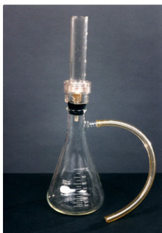
Figure 1. Nucleopore filter funnel assembly for concentrating water samples.
