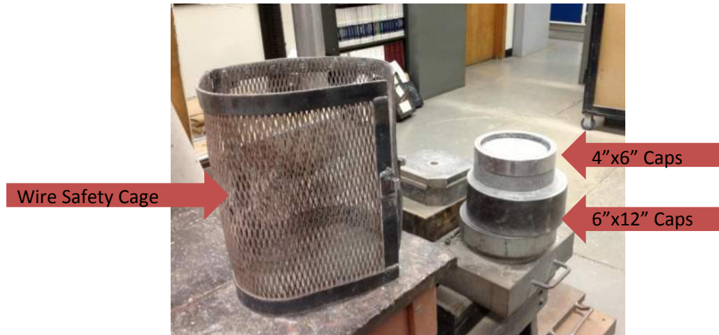
Figure 4. Wire Safety Cage and Test Caps
